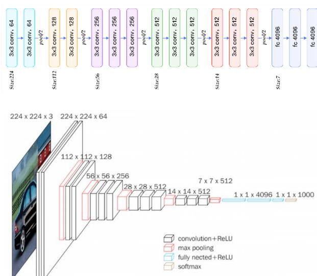
**Figure 3.** VGG16 neural network architecture
