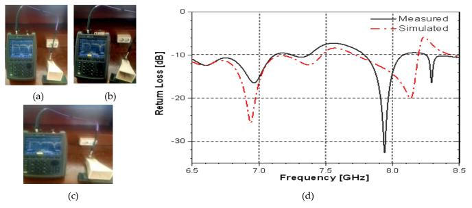
**Figure 14.** Laboratory Measurements and Comparision: (a) Horn Without CSLS Array; (b) Horn With CSLS Linear Array; (c) Horn With CSLS Triangular Array; (d) Comparision Between Simulation and Implementation Results.
