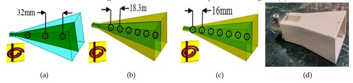
Figure 8. Horn Loaded With CSLS Linear Array: (a) Three Unit Cells; (b) Six Units; (c) Seven Unit Cells; (d) Fabricated.
