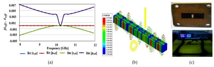
Figure 7. CSLS Linear Array Results: (a) Re. and Im. Parts of  $\epsilon$  and  $\mu$ ; (b) The E-Field [V/m]; (c) Laboratory Measurement.
