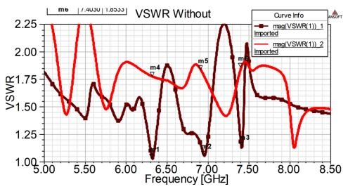
(b) VSWR (1)\_2,Horn Without Arrays; VSWR (1)\_1,Horn With Triangular Array
