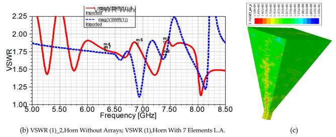
**Figure 9.** Horn Loaded Linear Array Results: (a) Comparision RL [dB; (b) Comparision VSWR of Horn Without CSLS and Loaded With Seven Elements Array; (c) CSLS Seven Elements Linear Array E-Field [V/m].
