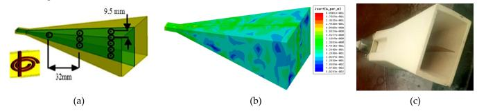
Figure 10. Horn Loaded With CSLS Triangular Array: (a) 3D View; (b) Electric Field Distribution [V/m]; (c) Fabrication.
