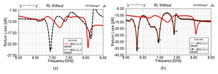
Figure 15. Horn Comarision Results: (a) Without and With 7-Elements Array; (b) Without and With Triangular Array
