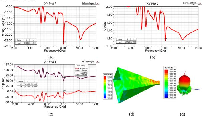
Figure 3. Horn Without CSLS Array Simulation Results: (a) RL [dB]; (b) VSWR; (c) Zin  $[\Omega]$  (d) Js[A/m]; (e) Radiation [dB]. Based on the simulation findings displayed in Figure 3, the suggested structure adds a matching antenna parameter of -24.19 dB return loss with 1.13 VSWR at the 53 ohm real component of the input impedance with a bandwidth of 6.44 GHz. The results presented in Table 2 are introduced by the proposed pyramidal horn.
