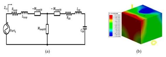
Figure 5. The CSLS Unit Cell: (a) Equivelent Circuit; (b) E-Field [V/m].
