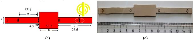
Figure 6. The CSLS Linear Array (a) Dimension [mm]; (b) Fabrication.
