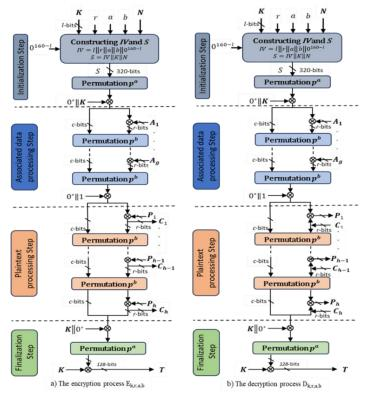
Figure 1. Ascon-128 encryption and decryption process.
