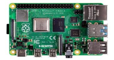
Figure .4. Raspberry Pi 4 Model B and its peripherals connections [6].
