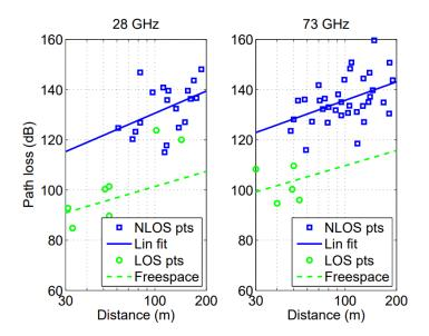
Figure 1. Scatter plot along with a linear fit of the estimated omnidirectional path losses as a function of the TX-RX separation [35].
